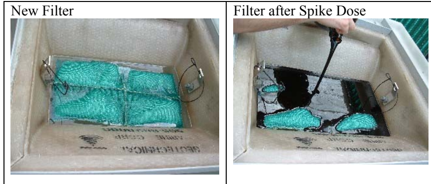
Figure 10. Photographs of Hydro-Cartridge™ During the Spike Dose Experiment.
