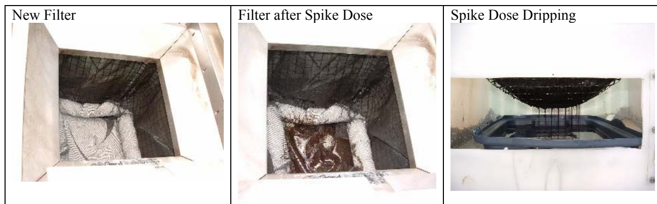
Figure 9. Photographs of FloGard+Plus™ During the Spike Dose Experiment.
