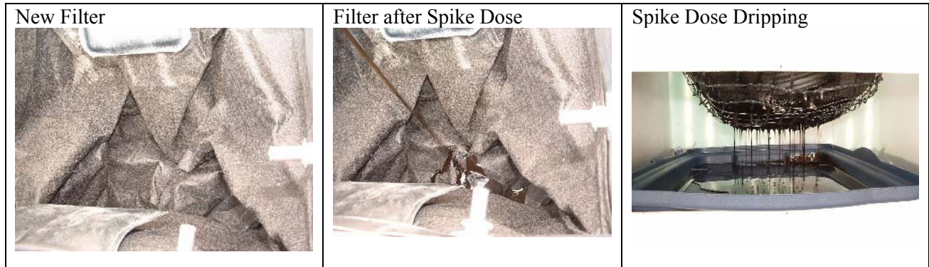
Figure 12. Photographs of Drain Pac™ During the Spike Dose Experiment.
