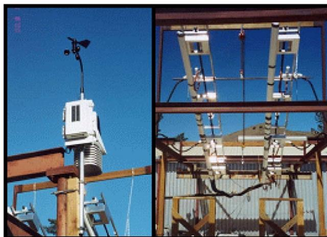
**Figure 3. Weather station and rainfall simulators.**
