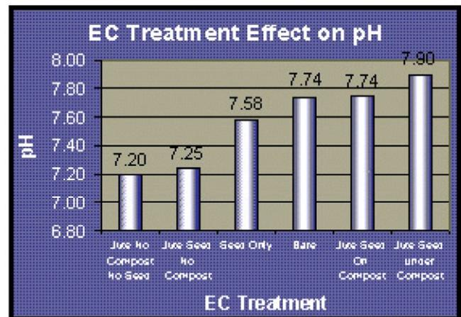
**Figure 7. EC treatment effect on pH levels.**
