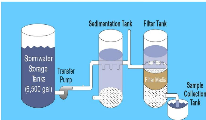
**Figure 2 Schematic of a Sedimentation/Filtration System**
