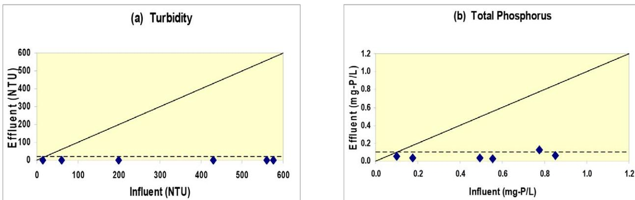
**Figure 7 Expanded shale filtration results for (a) turbidity and (b) total phosphorus (slow loading, submerged, following 24-hour sedimentation). (Dotted lines represent surface discharge limits and solid diagonal lines represent no treatment).**
