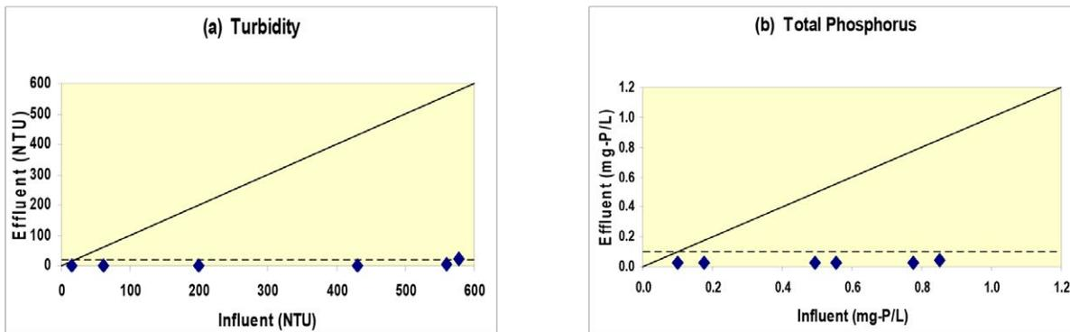
**Figure 6 Activated alumina filtration results for (a) turbidity and (b) total phosphorus (slow loading, submerged, following 24-hour sedimentation). (Dotted lines represent surface discharge limits and solid diagonal lines represent no treatment).**
