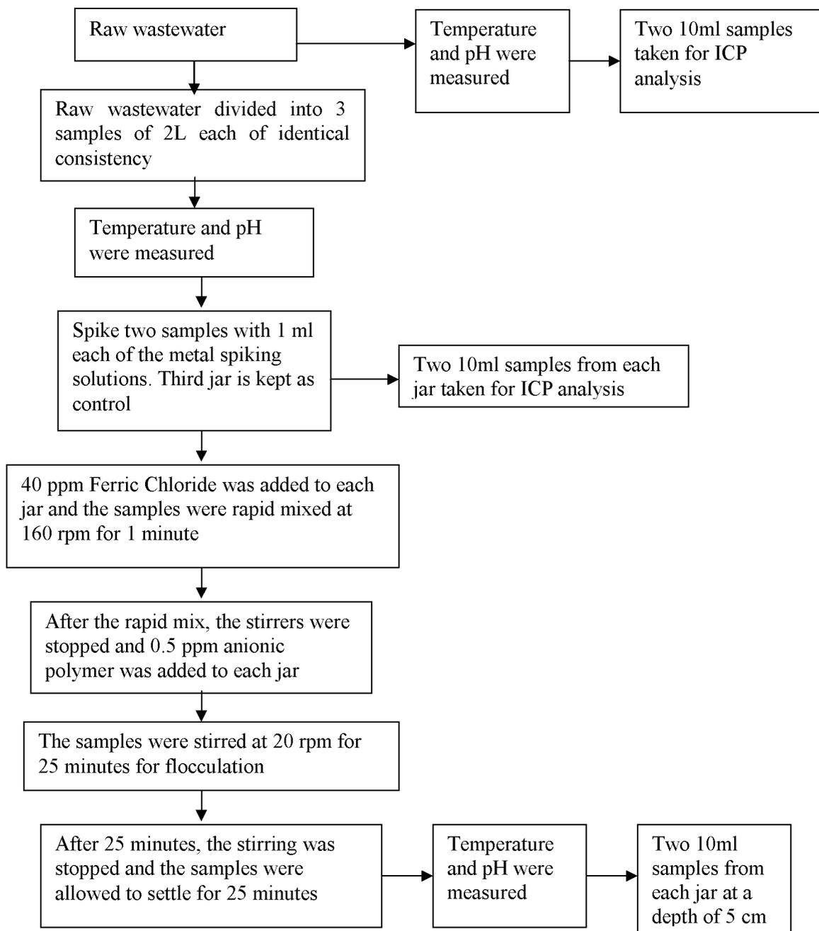
Figure 1—Flow chart procedure of jar test experiments (0.5 ppm = 0.5 mg/L).
